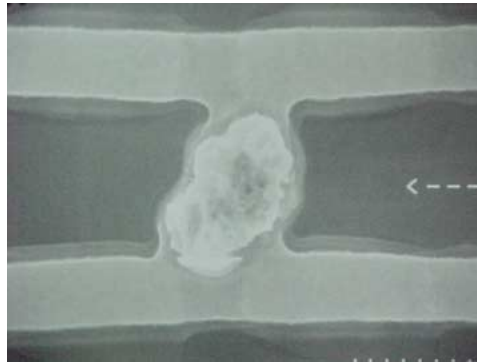
Photo 2-4 Dust-induced Wiring Short
