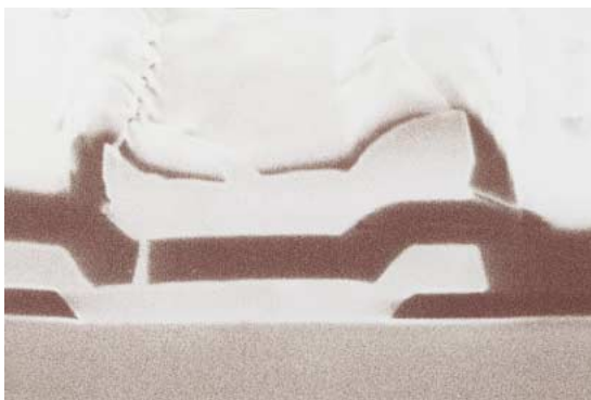
Photo 2-8 Cross Sectional View using FIB
