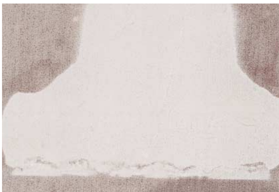
Photo 2-5 Cross Sectional View of Bonding Junction after Shelving at High Temperature
