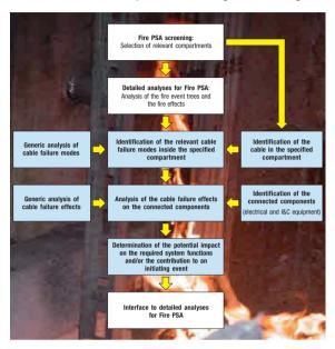
The FMEA-tool **CaFEA** (**C**able **F**ailure **E**ffect **A**nalysis) has been developed by GRS on the base of MS Access. **CaFEA** supports the analysis and records the result of the FMEA. The **CaFEA**-database contains
